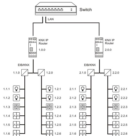
Fig. 2: KNX IP Router as a backbone coupler
