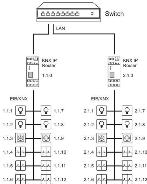
Fig. 1: KNX IP Router as a line coupler
