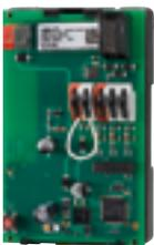
KNX RS485 Motor Controller which connects with the KNX bus to control a group of 1 to 6 similar Somfy RS485 motors.
