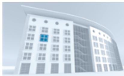
Within the same zone, all blinds behave the same way. Smaller zones enable more efficient and precise operation.
