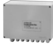
The Outside Sensor Box is the interface between the weather station, the Building Controller or Sub Controller. All measurement values are evaluated here and sent to the Building Controller. It requires an external 24 V AC/DC power supply.
