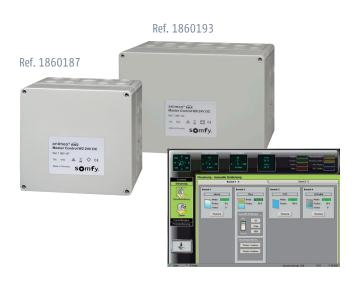
The animeo KNX Master Control W2/W8 V 3.0 is a building controller which enables a zone-based shadow management of 16 or more façade areas for a selection of 19 different types of blinds.
