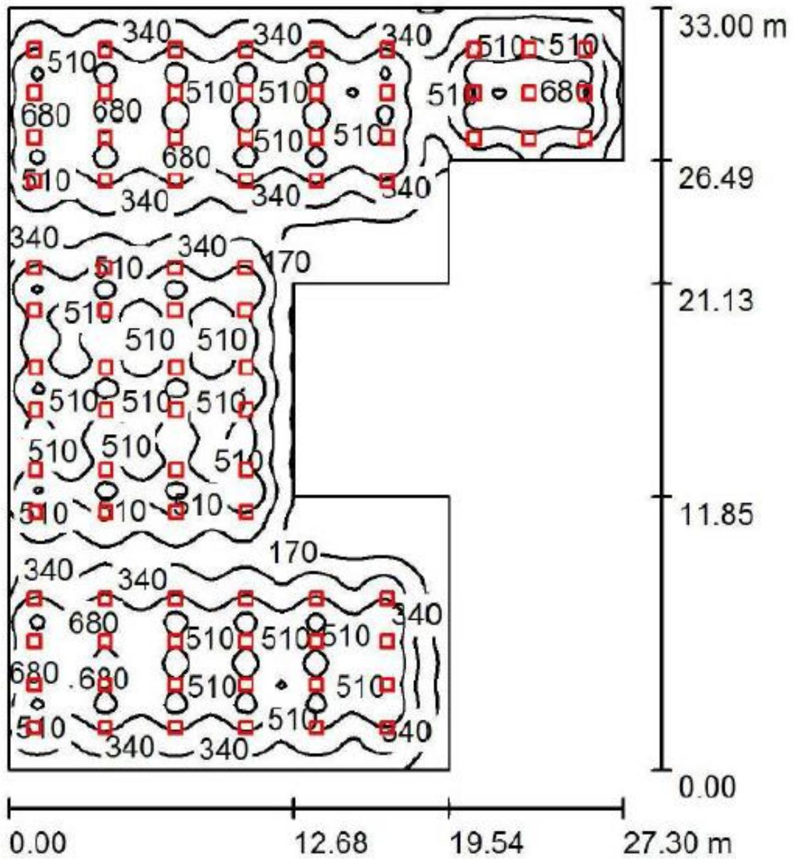
Figure 13 Lighting design model with 81 luminaries
