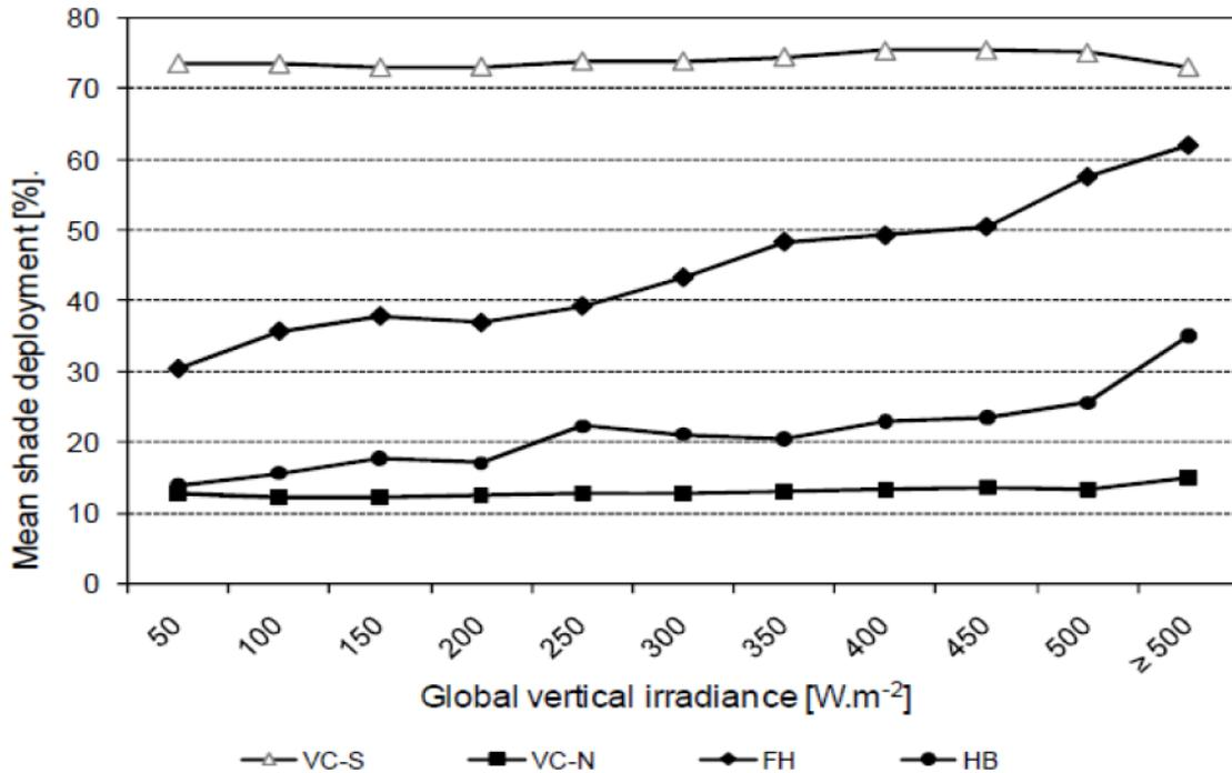
Figure 7 Percentage of shade deployment according to solar radiation
