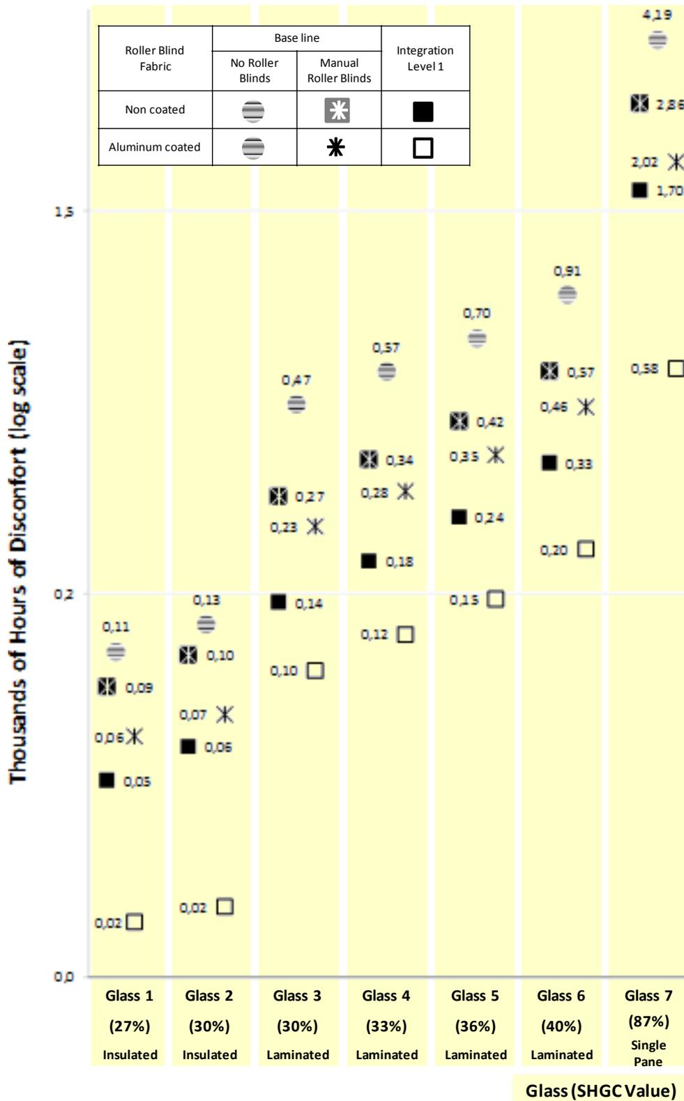
Figure 18 Thermal discomfort in degrees hour above 25°C in operating temperature
