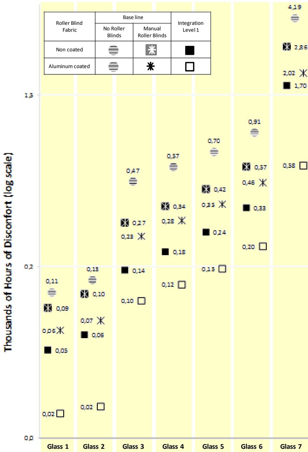
Figure 2 Thermal discomfort in degrees hour above 25°C in operating temperature.
