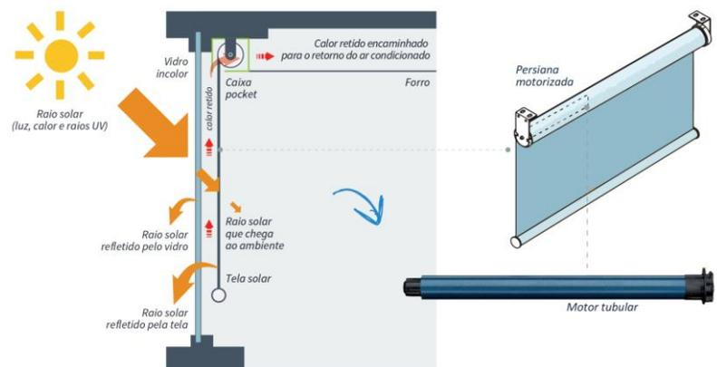
Figure 6 Interior shading installation
