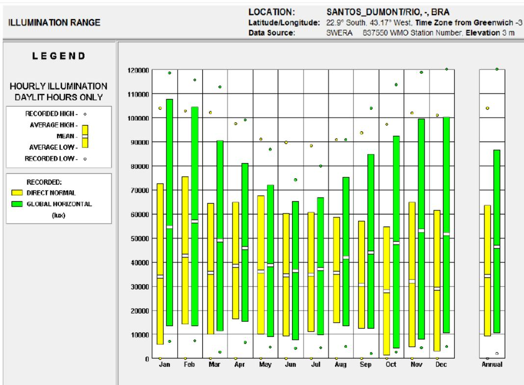
Figure 9 Direct and global illumination on a horizontal plane, hourly average [lux]
