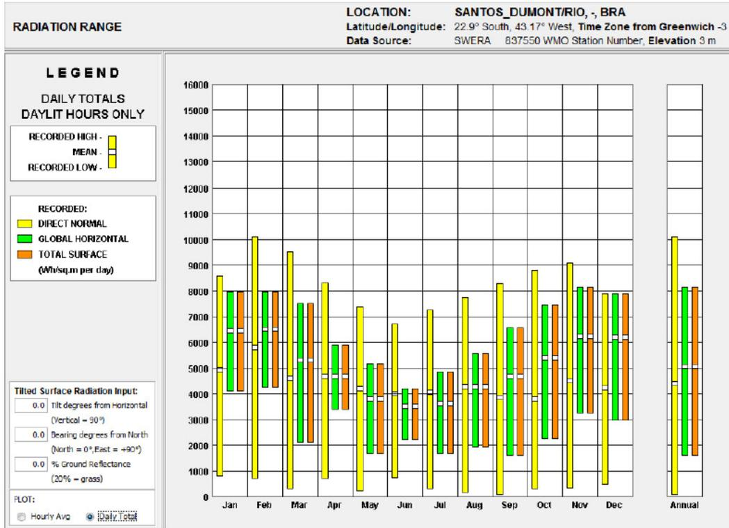
Figure 8 Direct and global solar radiation on a horizontal plane, total media a day [Wh / sf2]
